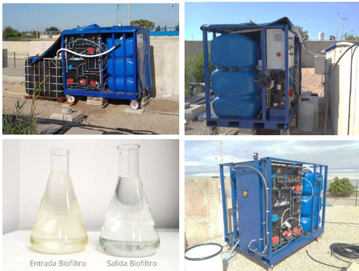
Figure 2: Images of the Biological Denitrification Pilot in the Mar Menor at 0.24 m 3 /h
